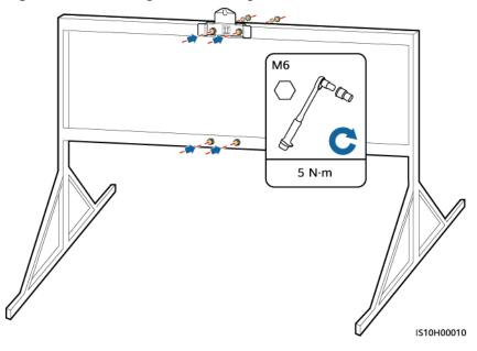
Figure 4-15 Securing the mounting bracket
