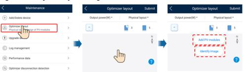
Figure 7-8 Physical layout design of PV modules
