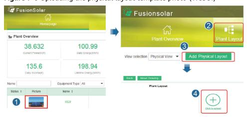
Step 2 Log in to https://intl.fusionsolar.huawei.com to access the WebUI of the FusionSolar Smart PV Management System. On the Homepage page, click the plant name to go to the plant page. Select Plant layout. Choose > Generate with AI, and create a physical layout as prompted. You can also manually create a physical location layout.
