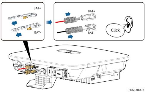
Figure 5-15 Connecting battery cables
