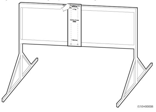
Figure 4-13 Determining the positions for drilling holes
