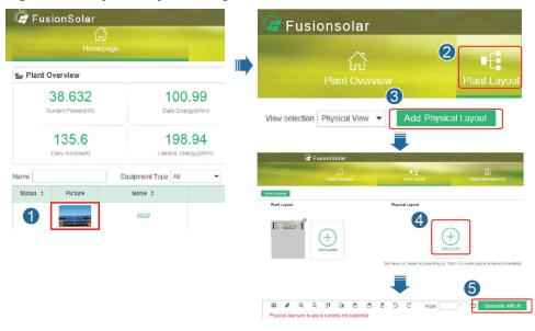
Figure 7-7 Physical layout design of PV modules
