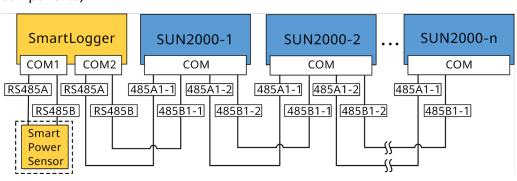
**Figure 5-20** SmartLogger networking (the dashed box indicates optional components)
